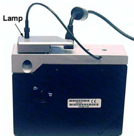
Figure 3. Plug the lamp into the top port for transmission.
