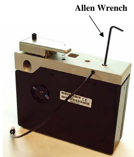
Figure 5. To remove the Leaf Probe from the Spectrometer, use an Allen wrench to remove the screws located on the top of the Leaf Probe.
