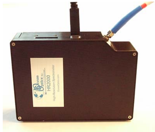
Figure 7. To use without the Leaf Probe, plug the fiber into the fiber port
