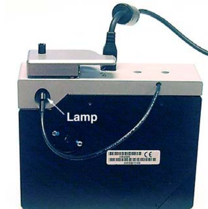
Figure 4. Plug the lamp into the side port measuring for measuring reflectance.
